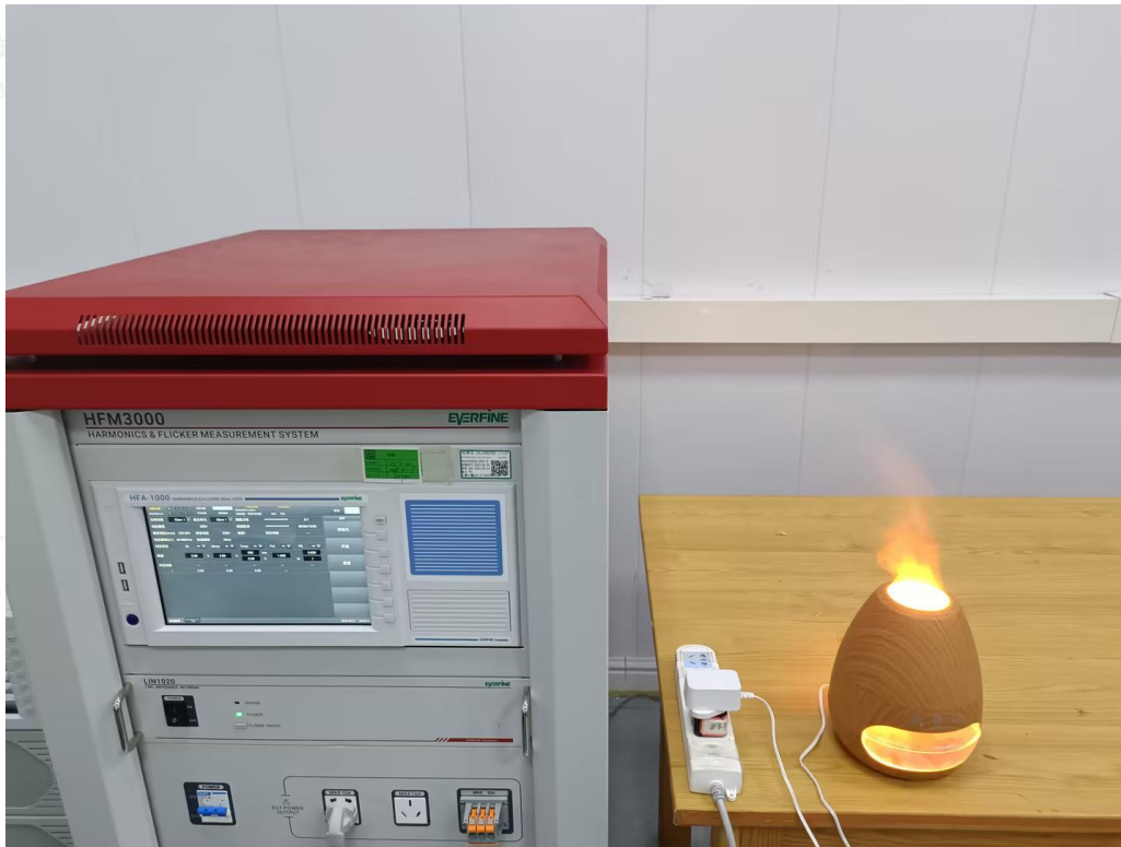
Photo of Harmonic & Flicker Measurement
